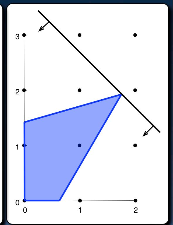
$$P := \left\{ x \in \mathbb{R}^2 : \begin{array}{c} x_1 + x_2 \le 3, \\ 5x_1 - 3x_2 \le 3 \end{array} \right\}$$
